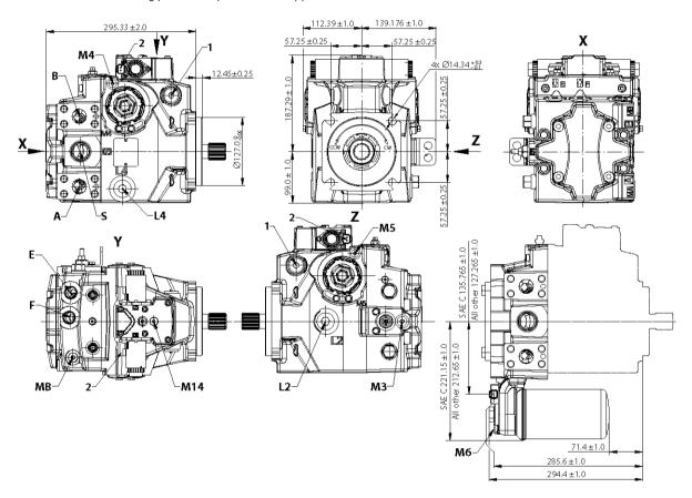
**A/B** system ports: Ø25.4 mm; M12 x 1.75; 20 min. full thread depth **MA/MB** (system), **M3, M6** (charge) gauge ports per ISO 11926-1:  $\frac{9}{16}$ –18 **M4, M5** (servo), **M14** (case) gauge ports per ISO 11926-1:  $\frac{7}{16}$ –20 **L2, L4** – Case drain ports per ISO 11926-1:  $\frac{15}{16}$ –12
